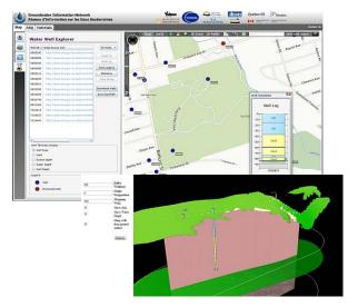
The GIN data analysis portal enables users to view water wells and supporting hydrogeological maps in 2D and 3D, and to display and download geological well logs and water information from wells. The GIN makes use of the GroundwaterML data transfer standard for water wells and GeoSciML to deliver the downhole geological information.
